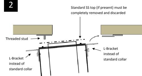
When bonding to worktop has cured <u>completely</u>, introduce S-Box<sup>™</sup> into rear slot and also front L-Bracket to its corresponding studs above.
