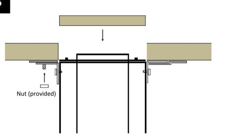
Tighten Nut onto threaded stud and centralise the S-Box<sup>™</sup> below its hole. The custom top may now be bonded to the lifting unit.
